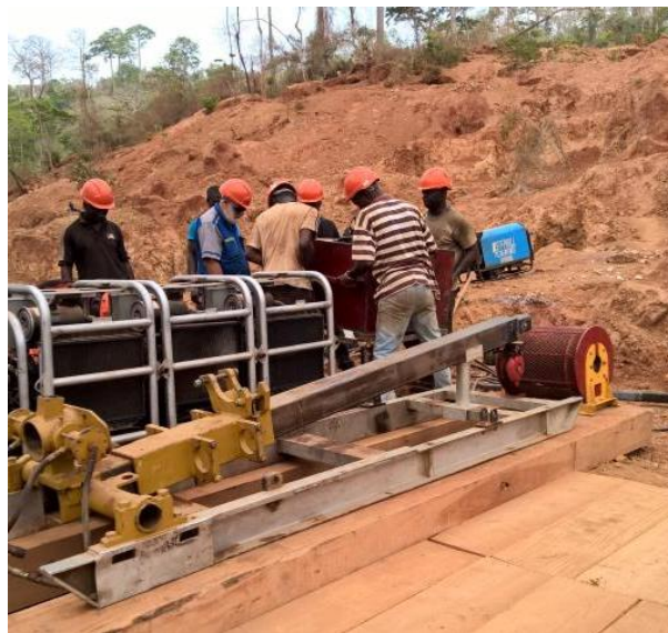
Figure 1: Portable diamond drill rig being set up on first drill site at Kokoumbo. Note large area of bedrock exposure in the background generated recently by artisanal miners.
